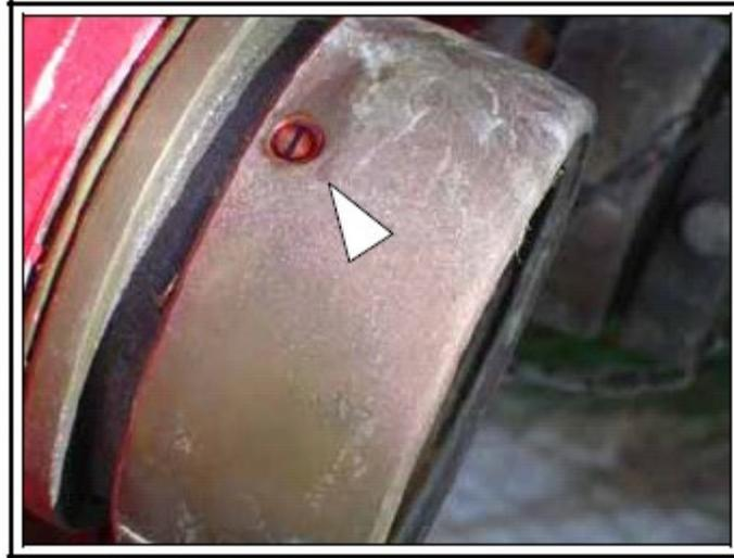
9. Drill out the slot of the set screw with a 1/4-inch drill bit until the slot is no longer visible. Check progresses several times so as not to drill through the set screw.
