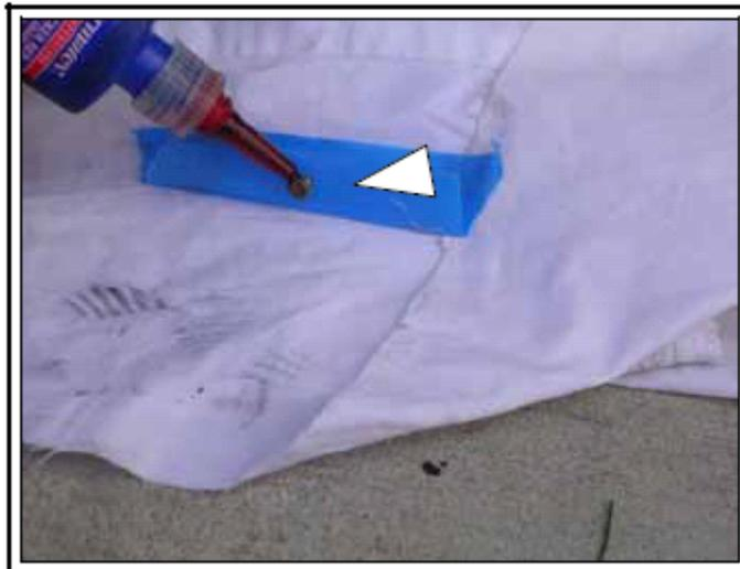
8. Replace the set screw flush with the casing and apply a small amount of red thread locker around the set screw. Allow to harden per manufacturer's directions.
